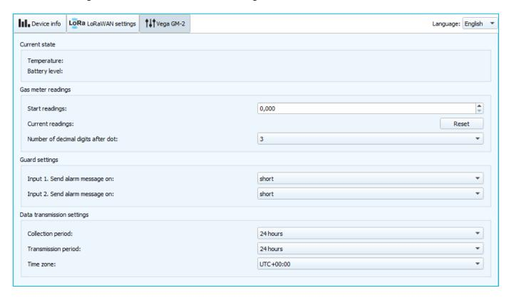
**Current state** – displays the current parameters of the device - the temperature and the battery level.
