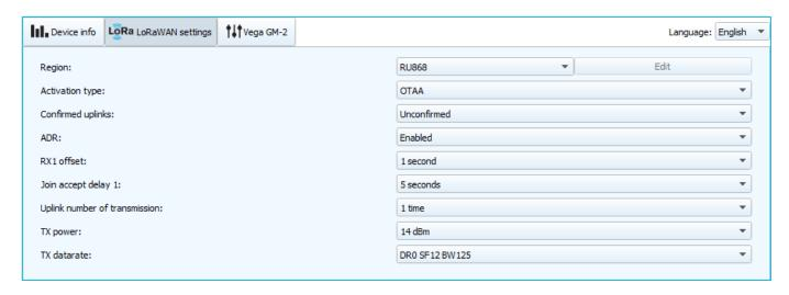
**Region** - allows you to select one of installed frequency plans or specify a custom frequency plan. Custom frequency plan is EU-868 based.
