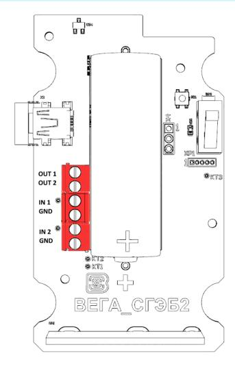
LoRaWAN modem has 2 security inputs. The device monitors its closure or opening, depending on the settings in the "Vega LoRaWAN Configurator" application. In the case of a security input triggering, the device is activated and sends an alarm message to the network.
