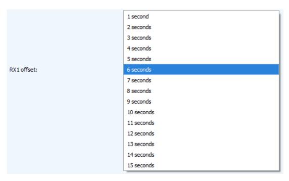
**Join accept delay 1** (not displayed in the "Simple" mode) – sets the time that the device will open the first receiving window to receive confirmation for the join request from the LoRaWAN network while OTAA mode active. The second window always opens after 1 second after the first.
