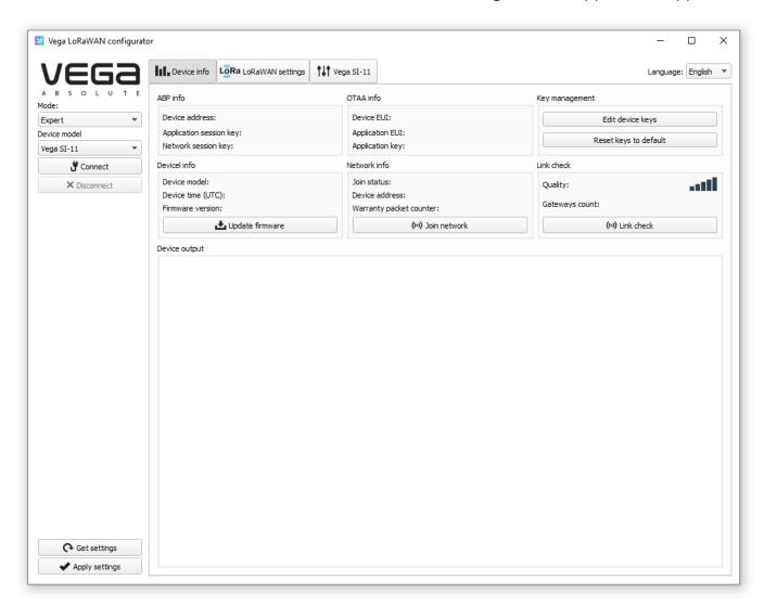
The menu on the left allows you to switch between the "Simple" and "Expert" modes, select the device model, connect to the device or disconnect from it, get and apply settings.
