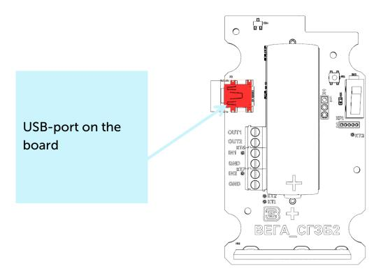
Before connecting the device to the computer for the first time, you must install the driver for the COM port stsw-stm32102, which can be downloaded from iotvega.com. After running the executable file VCP\_V1.4.0\_Setup.exe, the installer window will appear:
